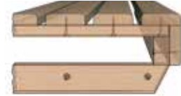
8. Supporting lath, screwed.
