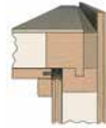
3. Wall to ceiling connection with deep-groove joint.
