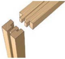
4. Frame with double-groove, double-tenon joints for optimum stability.
